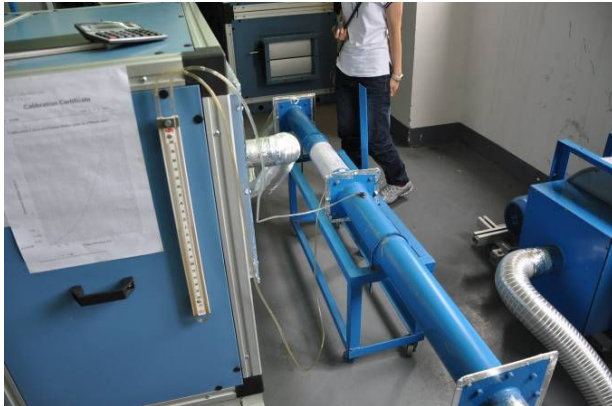
Air Leakage Test Demonstration
